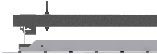
1 Hook-On Panel 2 J-Profile 3 Primary Channel 4 Hanging System 5 Perimeter Wall Angle 6 Allure Panel
